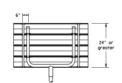
Use Extruded Alum. Windbeam as stiffeners See SMD (2-1) for additional details
